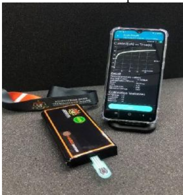
Figure 2. A portable electrochemical reader with inserted SPCE (right) and a mobile phone unit (right).
